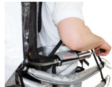
Hand operated Air Pump as pressure equipment
